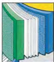
Suitable for agglomeration of small water vapor and oil mist, can filter up to 0.01 microns of aggregates (0.001ppm maximum residual oil content)
