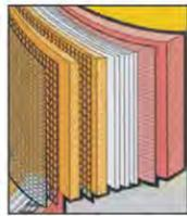
Suitable for removing large amounts of liquid and 0.01 microns of aggregates (0.01 ppm maximum residual oil content)
